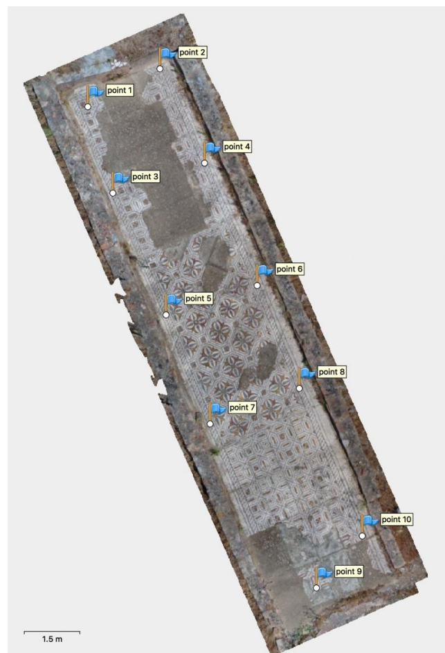
Figure 6. Position of the ten ground control points used to geometrically correct the unmanned aerial vehicle (UAV) mosaic survey.
